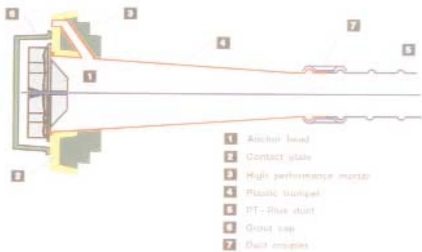
With the press release of September 25, 1992, the British Department of Transport is banning grouted post-tensioning for new construction. The main area of concern is corrosion of the prestressing steel resulting from improperly grouted tendon ducts.
