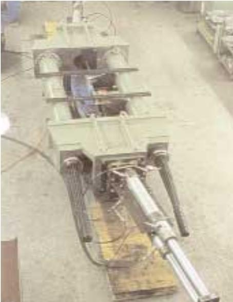
a long-term load test was carried out by keeping the load constant at 40 % of the nominal breaking load over a period of 11 days, in order to determine the creep behaviour of the material.
