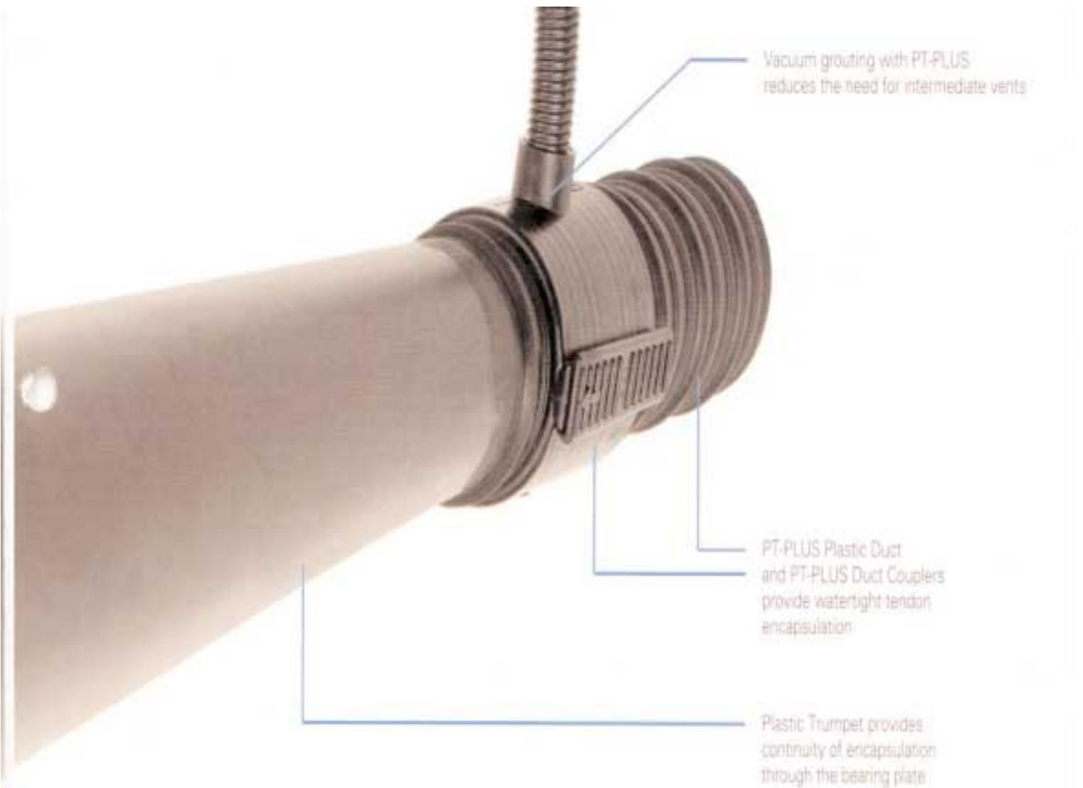
Vacuum grouting with PT-PLUS reduces the need for intermediate vents
