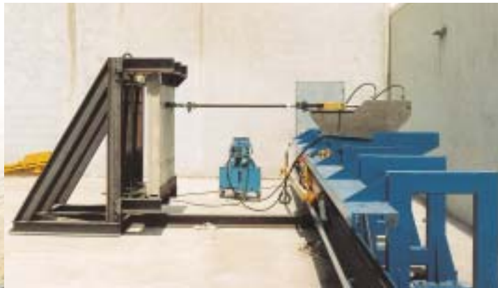
Clevis connector pullout test.
