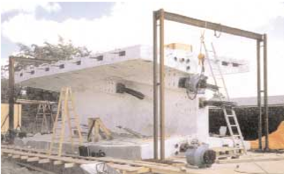
European Strobaelt Group verified VSL's blister design model with full-scale testing.
