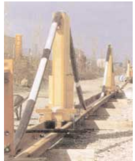
Testing program was performed on tendons up to 70m in length
