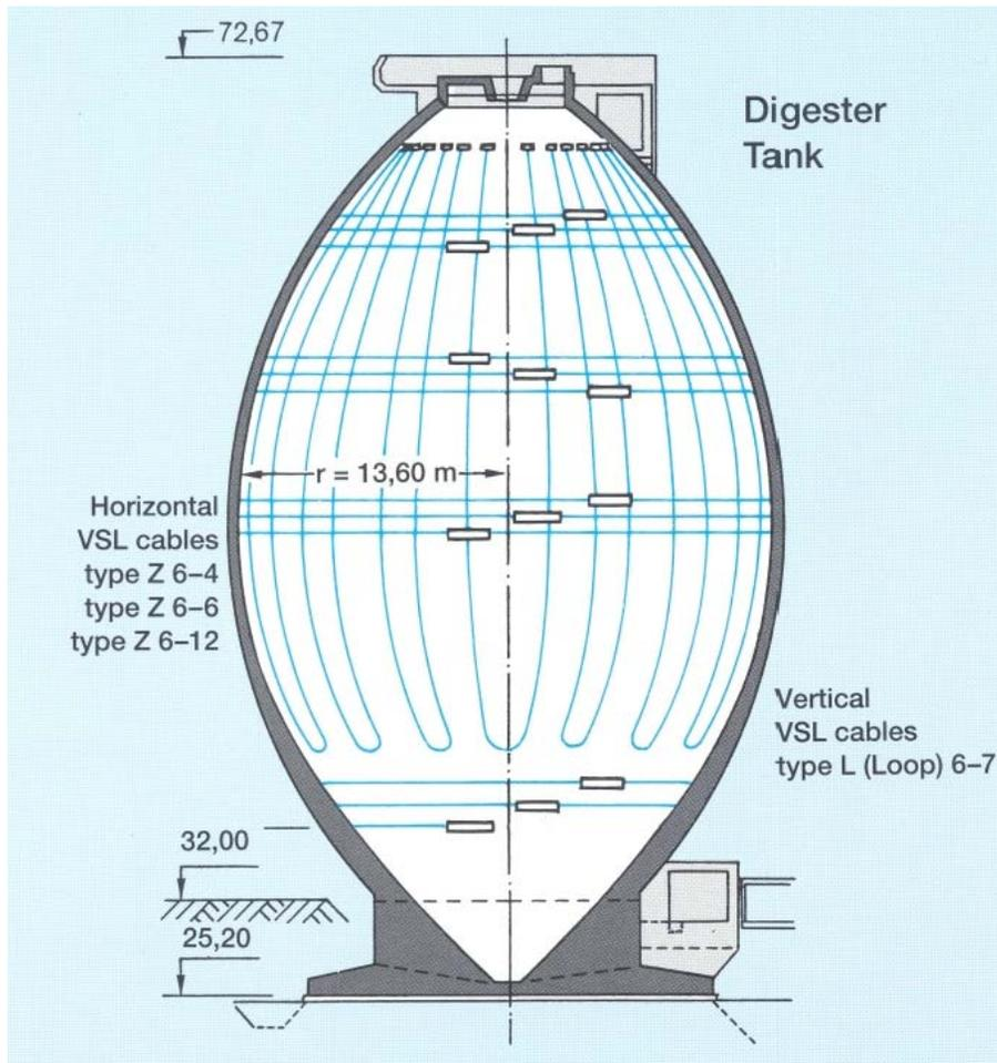
completed and the formwork was jacked upward, exposing the anchorage blockouts in the concrete below, the post-tensioning strand was pushed through the duct with specially designed VSL equipment. To facilitate the construction schedule even further, the tendons were stressed only after all concreting was completed. Upon completion of stressing, the tendons were grouted and the blockouts were filled with concrete to provide a smooth and continuous shell surface.
