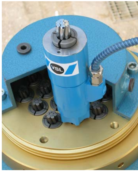
▲ The new VSL monostrand load cell installed on model
